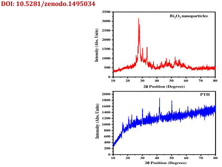
Fig. 2. XRD pattern of Bi<sub>2</sub>O<sub>3</sub> nanoparticles and polythiophene (PTh)
