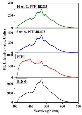
Fig.3. PL emission spectrum for Bi<sub>2</sub>O<sub>3</sub>, PTh, 5 wt % Bi<sub>2</sub>O<sub>3</sub>-PTh and polythiophene and 10 wt % Bi<sub>2</sub>O<sub>3</sub>-PTh composites
